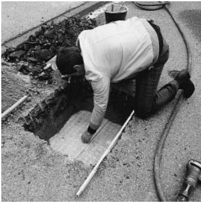
Fig. 6 Styropor foam board for frost protection in road construction. Samples taken 11 years after installation. The Styropor foam panels were in the same condition as that in which they were installed.
